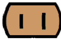
North American electrical outlet without ground (polarized)
